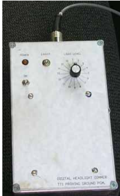
Figure 14. Photo. Headlamp controller box.
